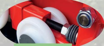
Tensioning of the tracks with a standard tool
