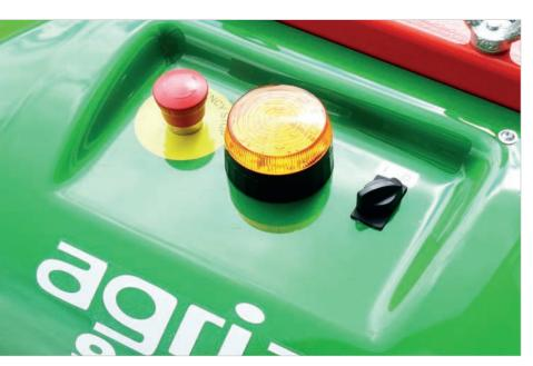
Both the machine itself and the remote control have an emergency **shut-off switch**, which stops the machine immediately when pressed.
