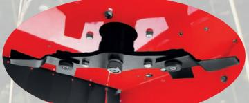
Fine result of cutting due to specially formed mulching blades made of hardened steel
