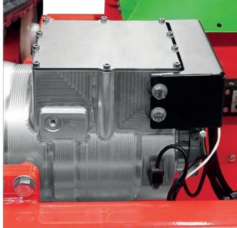
Say goodbye to cleaning and replacing carbon brushes because the electric motors and the generator are **brushless** and therefore **maintenance-free**.
