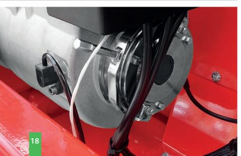
**Electromechanical Fail Safe Brakes** are mounted on both electric motors. These ensure maximum safety even on steep slopes and can be unlocked manually.
