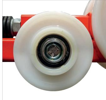
The robust **polyamide rollers** are equipped with two bearings each, filled with grease and sealed against dirt and moisture.
