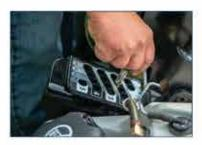
SINGLE-POINT HEIGHT-OF-CUT Operators can quickly and accurately change the cut height by simply adjusting the pin and raising or lowering the deck.
